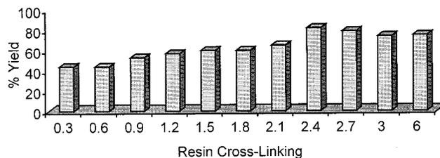
**Figure 1.** Relationship between the crude yield of the polymerization reaction and cross-linking of the solid support.
